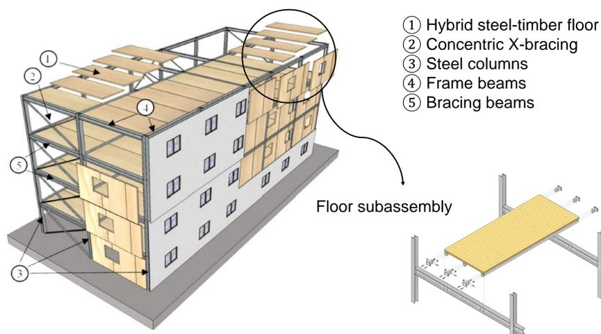
Figure 1. Hybrid construction system [1]
