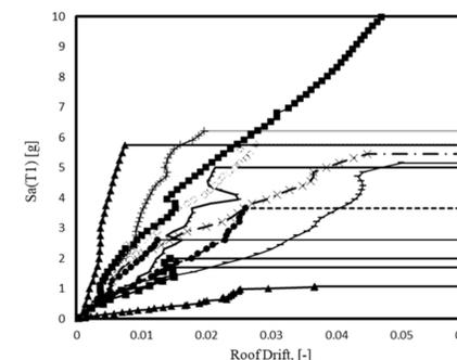
Figure 2. IDA curve for ground motion records
